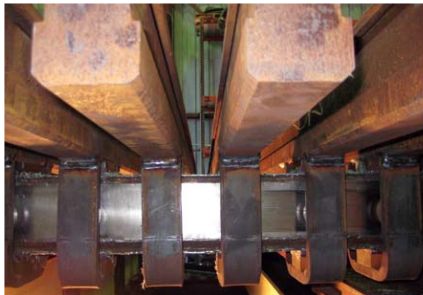
Figure 17 - Elevation view underneath showing the yoked connection to the support bar.
